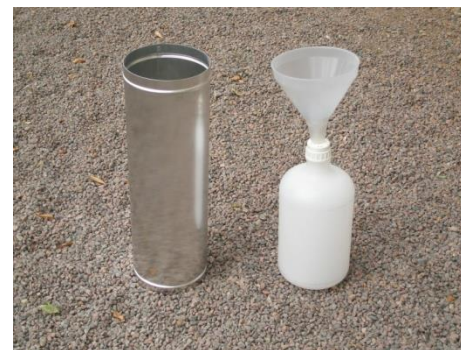
New bulk collector
